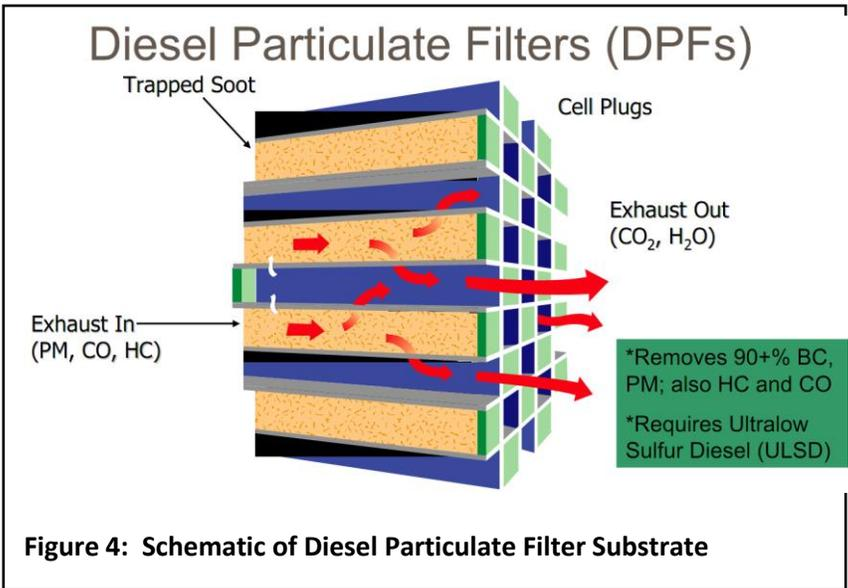
**Figure 4: Schematic of Diesel Particulate Filter Substrate**
